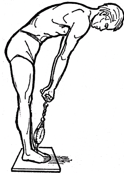
Figure 10. Measurement of the force by a steel dynamometer
